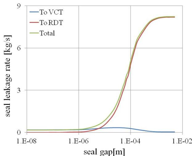
Fig. 3. Seal leakage rate with seal gap
