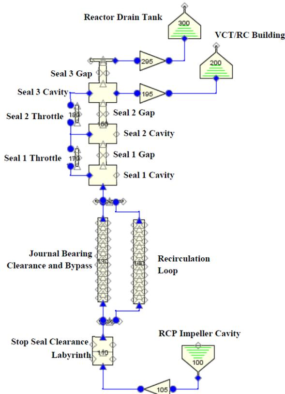
Fig. 2. RCP seal leakage RELAP5 nodal diagram
