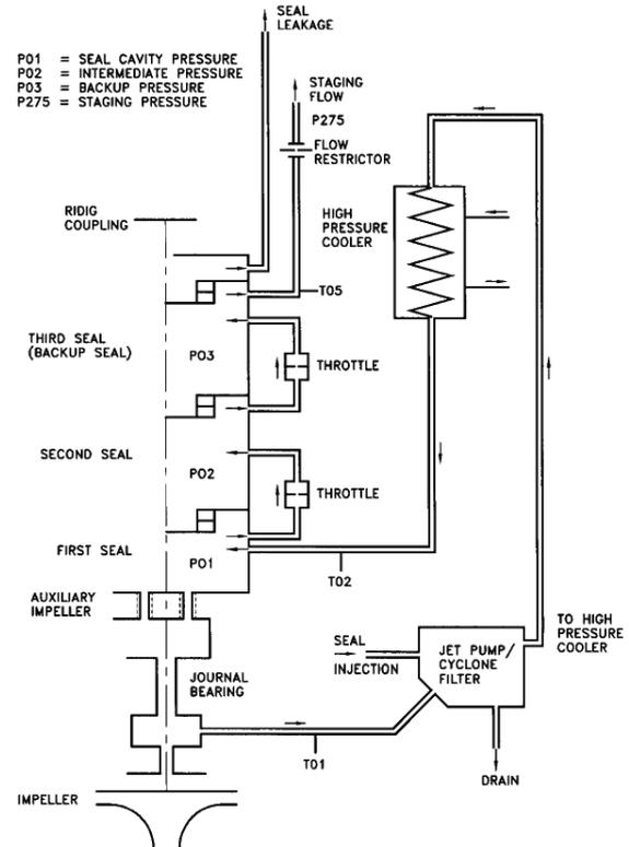
Fig. 1. the schematic diagram of KSB RCP seal
