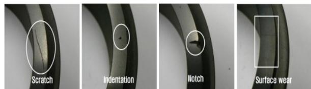
Fig. 3. Test specimens for defect tests
