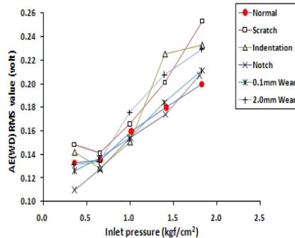
Fig. 6. RMS of AE signal with 50 kHz high-pass filtering
