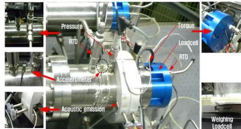
Fig. 2. Sensor locations on the mechanical seal housing
