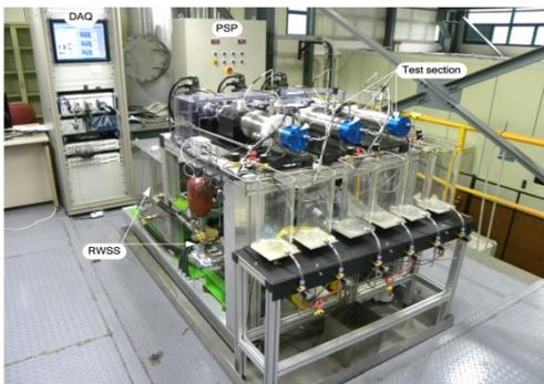
Fig. 1. Facility for mechanical seal experiment
