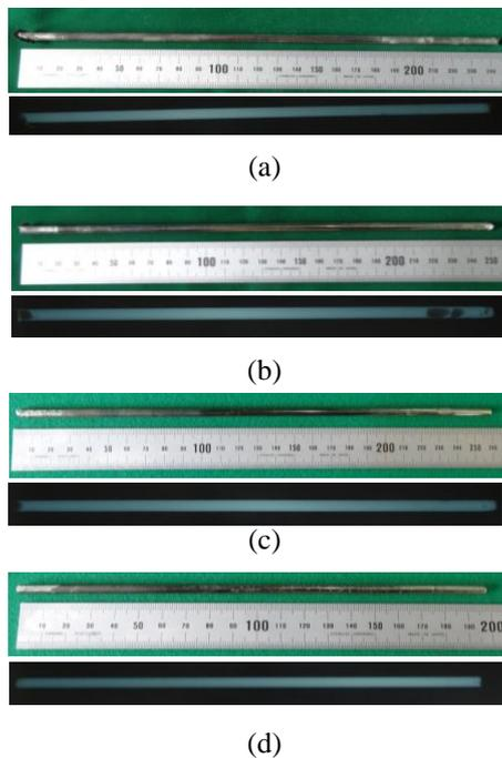
Fig. 2. Photographs and gamma radiographs of the U–Zr and U–Zr–Mn fuel slugs fabricated by injection casting under various casting conditions: (a) test a, (b) test b, (c) test c, and (d) test d
