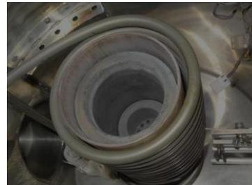
Fig. 1. Induction copper coil used for heating the raw materials.
