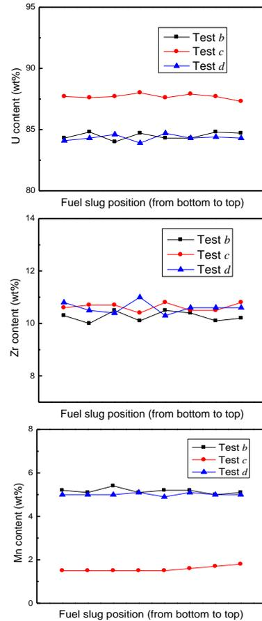
Fig. 3. Variations of chemical composition according to the position of a U–Zr–Mn fuel slug fabricated under different injection casting conditions: (a) U, (b) Zr, and (c) Mn
