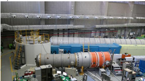
Fig. 1. Photos of current DC-TOF. The white big structure is fight tank for DC-ToF. The two cylinders are detector tank for other instruments : 40M-SANS and 18M-SANS
