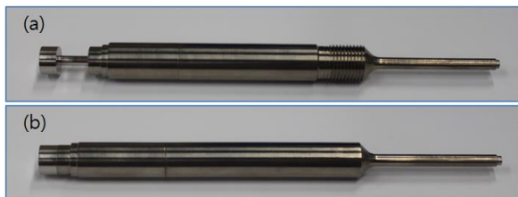
Fig. 4. LVDT core assembly (a) For fuel displacement measurement (b) For cladding tube length deformation measuring
