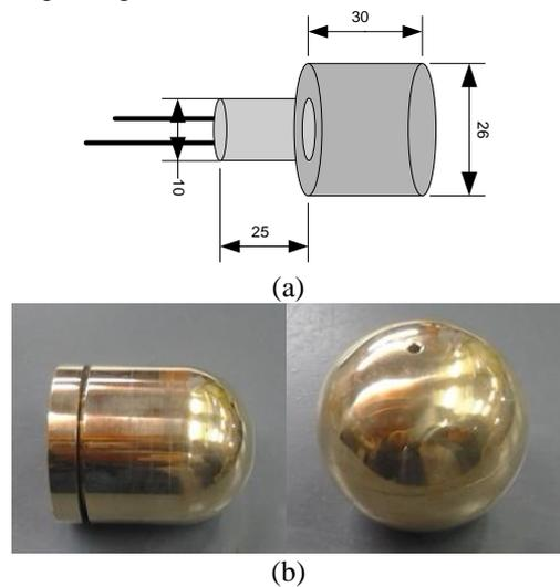
Fig.1. (a) Geometry of cylindrical heater (unit mm)
