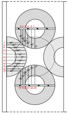
Fig.3. Schematic of locations of temperature measuring point
