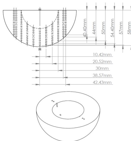
Fig.2. Schematic of the fabrication of temperature measuring point
