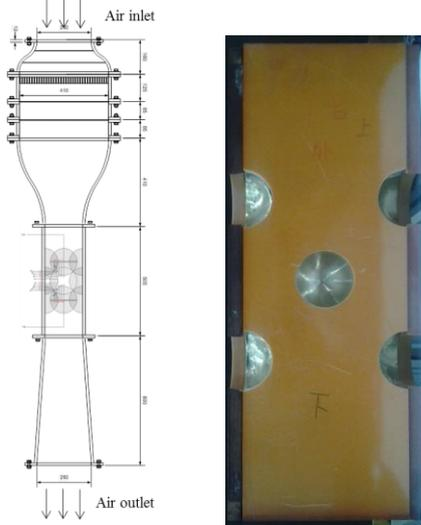
Fig.4. Schematic of wind channel (left) and test section (right)
