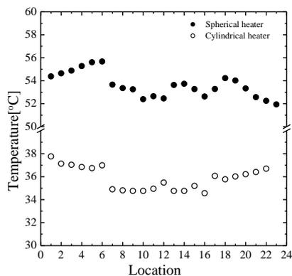
Fig.5. Comparison of the thermal field in terms of using different shapes of heater
