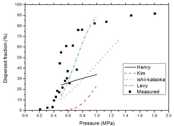
Figure 11. Comparison for Surry Cavity (hole diameter = 9.53mm)
