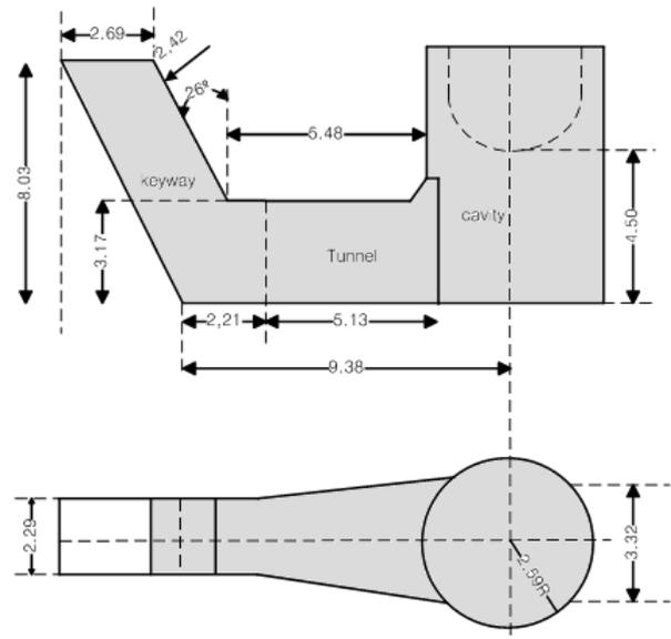
**Figure 3.** Zion 1/10 cavity model
