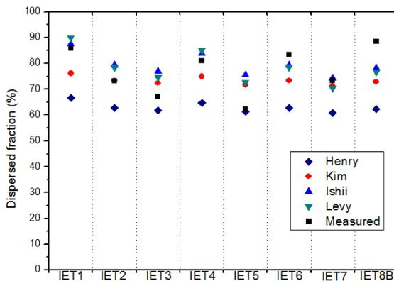
Figure 13. Comparison for Zion Cavity (hole diameter = 3.5mm)
