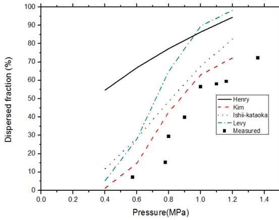
Figure 7. Comparison for Kori 1&2 Cavity (hole diameter = 20mm)
