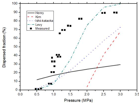
Figure 12. Comparison for Surry Cavity (hole diameter = 4.76mm)
