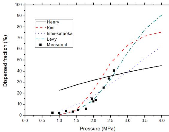
Figure 8. Comparison for YGN 3&4 Cavity (hole diameter = 10mm)
