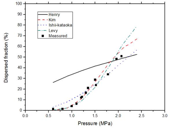
Figure 9. Comparison for YGN 3&4 Cavity (hole diameter = 15mm)
