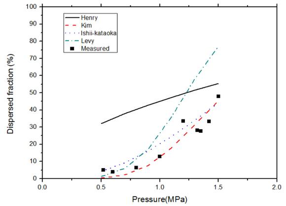
Figure 10. Comparison for YGN 3&4 Cavity (hole diameter = 20mm)
