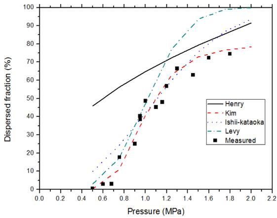
Figure 6. Comparison for Kori 1&2 Cavity (hole diameter = 15mm)
