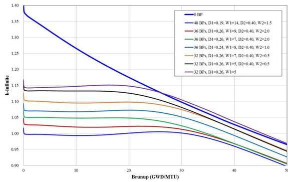
Fig. 6. Infinite Multiplication Factors of Double Layer BP ( $B_4C/Gd$ ) vs. Burnup
