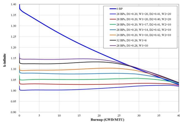
Fig. 7. Infinite Multiplication Factors of Double Layer BP ( $B_4C/B_4C$ ) vs. Burnup
