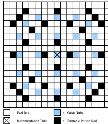
Fig. 9. Cross Sectional Drawing of 17x17 WH Type FA (A0)
