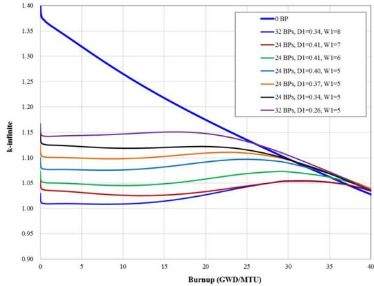
Fig. 5. Infinite Multiplication Factors of Single Layer BP ( $B_4C$ ) vs. Burnup
