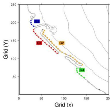
Fig. 7. The group of wave height sampling points (G1:front of intake, G2:front of breakwater, G3:left side of breakwater, G4:right side of breakwater) [7]
