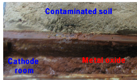
Fig. 1. Metal oxides generated in the cathode chamber
