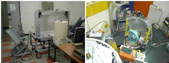
Figure 4. Functional test of the curved two-dimensional position-sensitive neutron detector at the laboratory and installation at the four circle diffractometer at HANARO research reactor.
