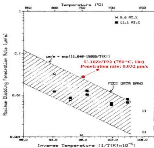
Fig. 4. Maximum eutectic penetration rate along cladding direction.
