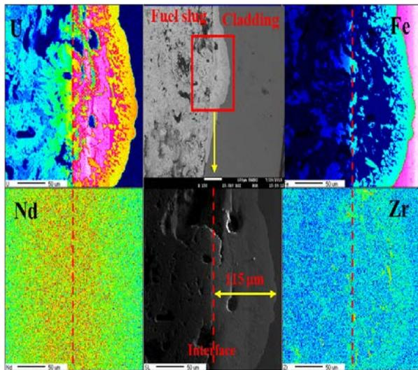
Fig. 3. Constituent distributions and eutectic penetration depth of U-10Zr/T92 specimen after heating test (750 °C, 1 hr).
