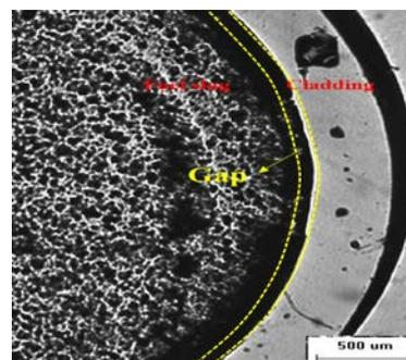
Fig. 2. Microscope photograph of U-10Zr-5Ce/T92 specimen after heating test (800 °C, 1 hr).
