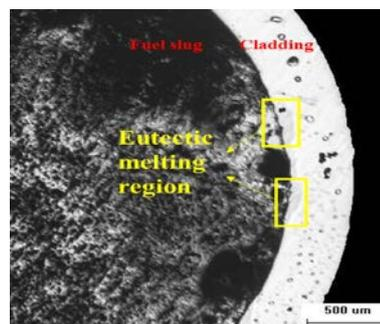
Fig. 1. Microscope photograph of U-10Zr/T92 specimen after heating test (750 °C, 1 hr).
