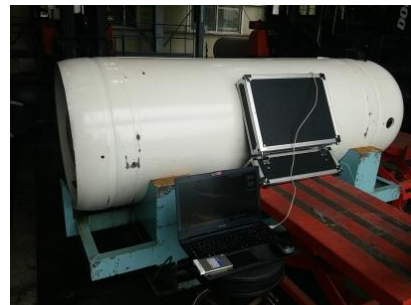
Fig. 3. Experimental setups and data acquisition for the verification of UF 6 cylinder at the KEPCO Nuclear Fuel (KNF).
