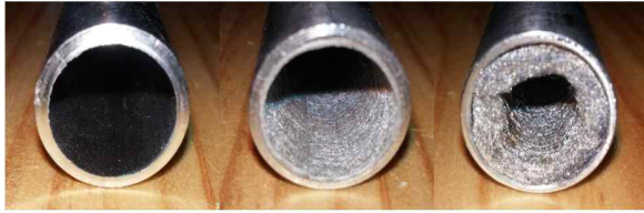
Fig.3 Manufactured wick structures of heat pipes
