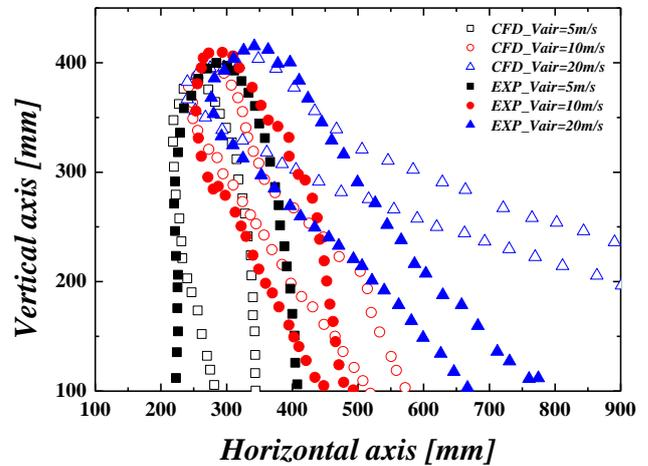
Fig. 3. Deformation of the liquid film spreading profile in the case of 0.5 m/s ECC injection velocity
