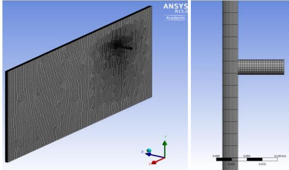
Fig. 2. Numerical mesh of 1/20 scaled plate DVI
