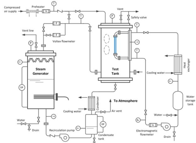
Fig. 1. Condensation experiment facility
