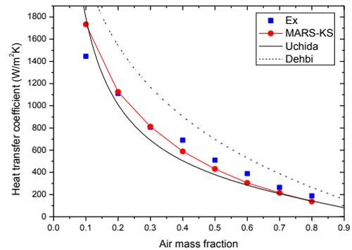
Fig. 4. Comparison result at 4 bar
