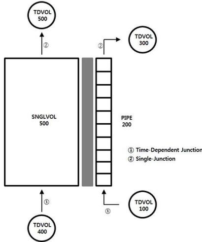
Fig. 2. Test tank Nodalization for MARS-KS
