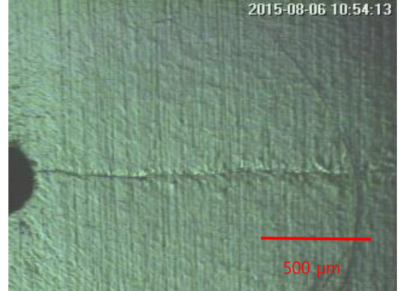
Fig. 15. Picture of crack with travelling microscope
