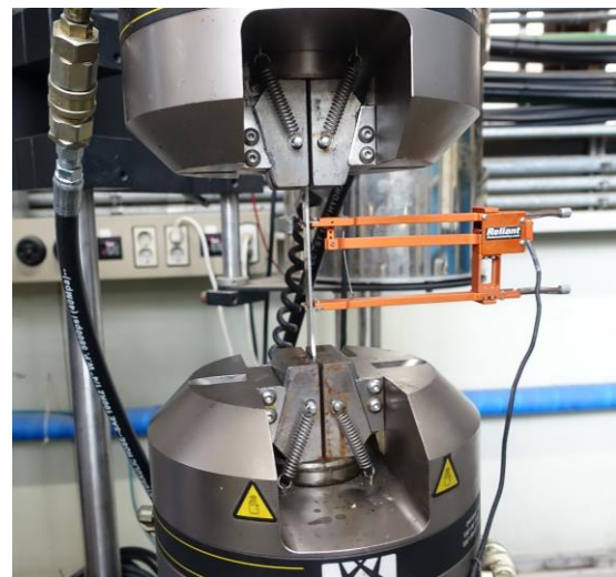
Fig. 2. Tensile testing of Type 304 stainless steel
