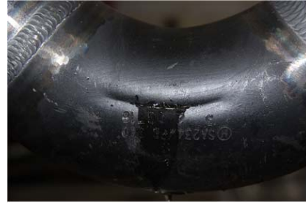
Fig. 6. Ultimate failure state of elbow specimen: penetration crack & leakage of water at the crown of elbow.
