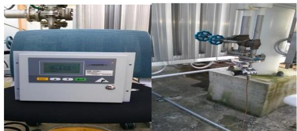
Fig 3. Oxygen sensor connected to the V-8 valve
