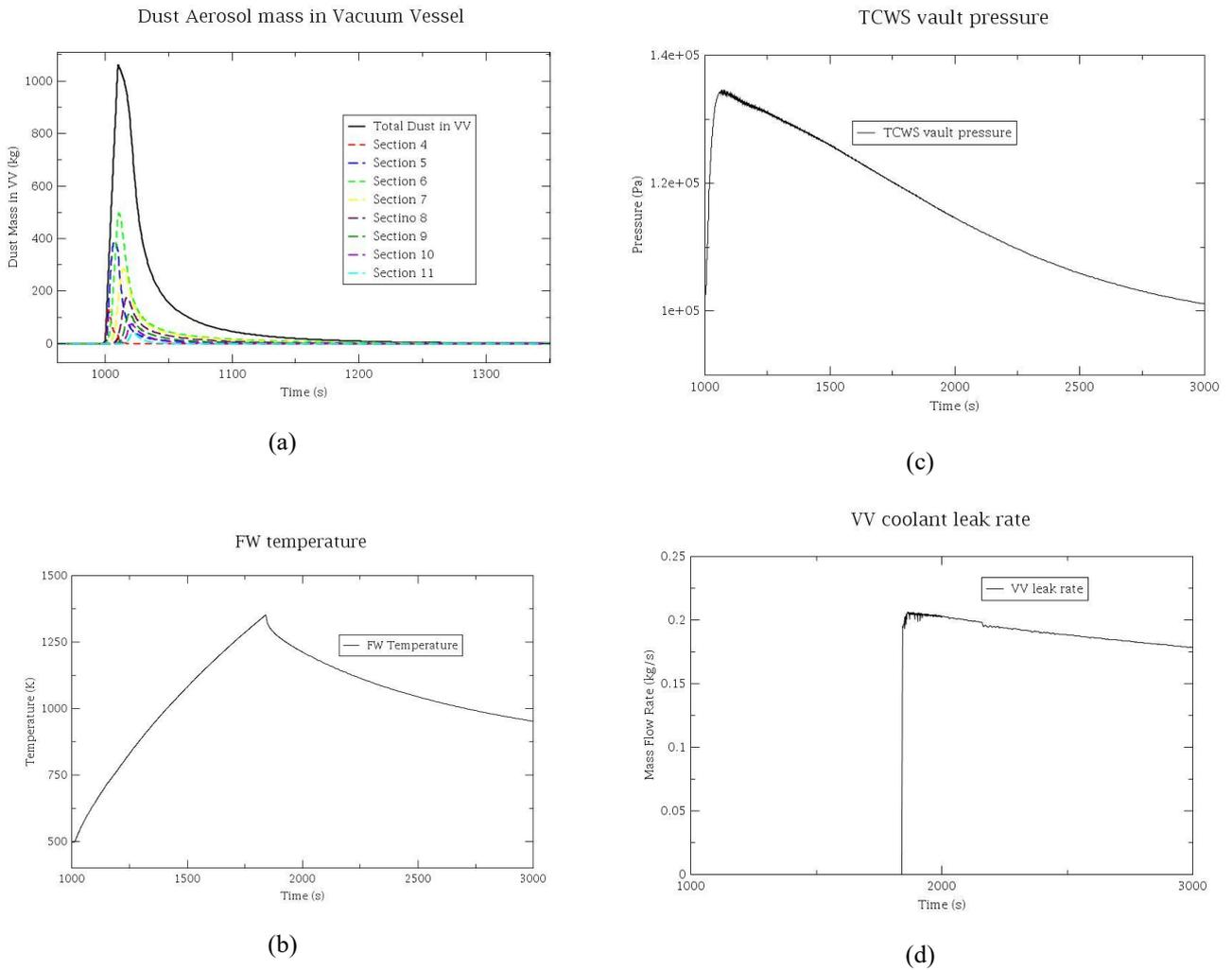
Fig. 2. The result of Fusion Power Termination System Failure accident analysis
