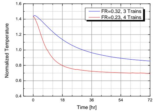
Fig. 2. Temporal behavior of temperature of the RCS
