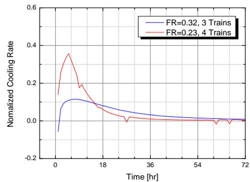
Fig. 3. Temporal behavior of cooling rate of the RCS
