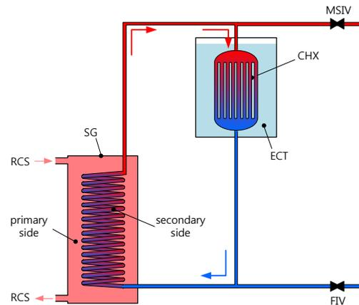
Fig. 1. The schematic of the PRHRS
