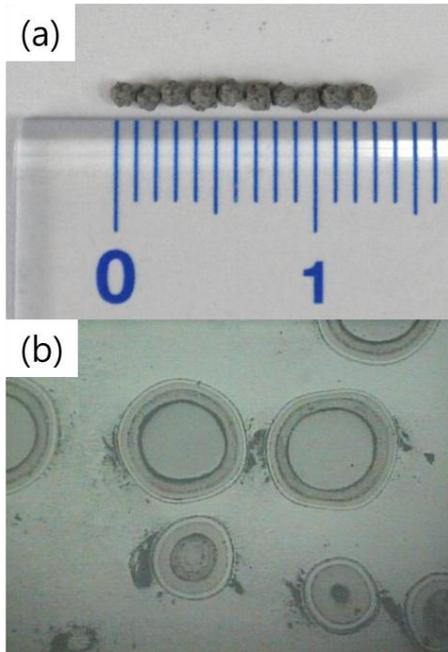
Fig. 1. (a) Image of powder overcoating TRISO particles, (b) Optical microscope image of FCM pellets.
