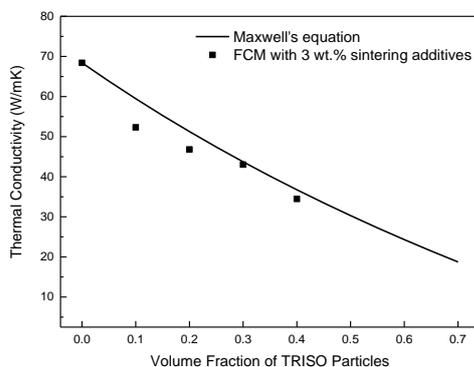
Fig. 3. Measured thermal conductivity of FCM pellets with different volume fraction of TRISO particles and the prediction of Maxwell's equation
