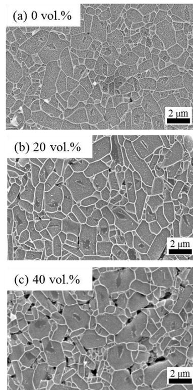
Fig. 2. SEM micrographs of etched surface of FCM pellets with TRISO particles of (a) 0 vol.%, (b) 20 vol.% (c) 40 vol.%
