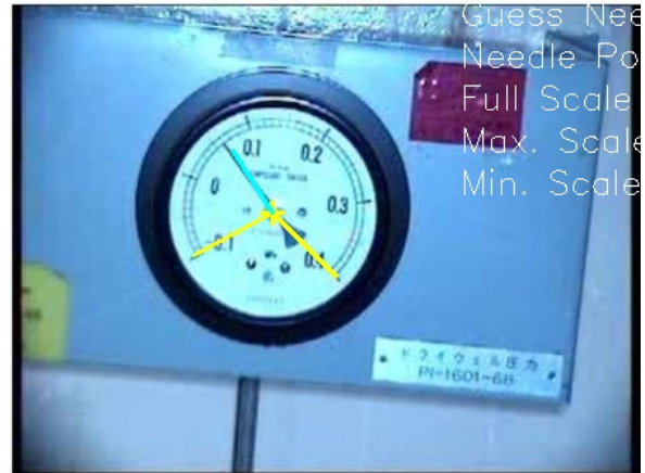
Figure 5. Recognition of the D/W (dry well) pressure
