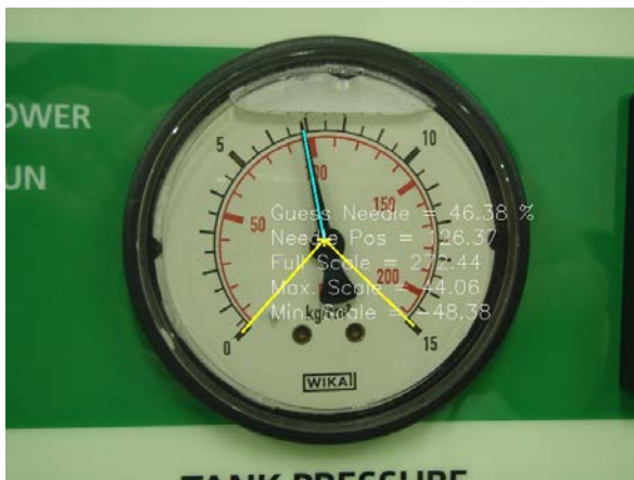
Figure 4. Reading result of the pressure gauge
