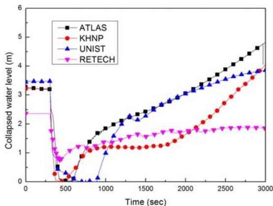
Fig. 6. Pressurizer water level for APR1400
