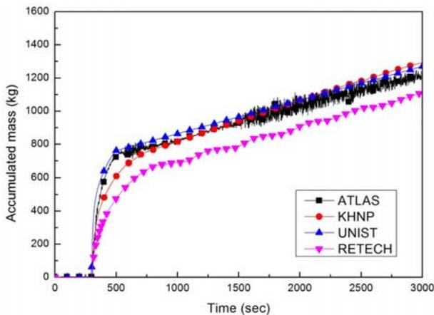
Fig. 1. Accumulated mass from the break flow for ATLAS
