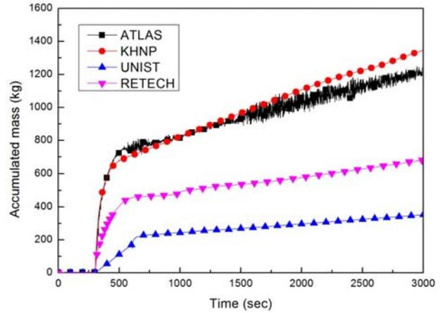
Fig. 2. Accumulated mass from the break flow for APR1400
