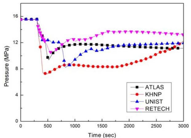
Fig. 4. Pressurizer pressure for APR1400
