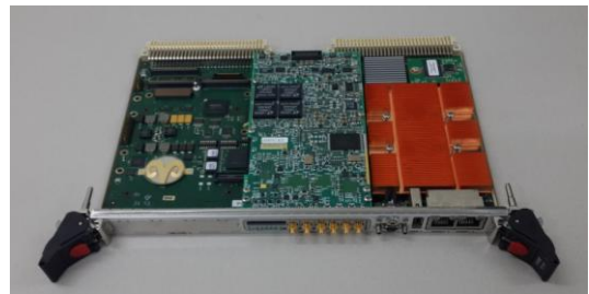
Fig. 3. IVME7210 baseboard and Pentek7156 FPGA PCI PMC extended board
