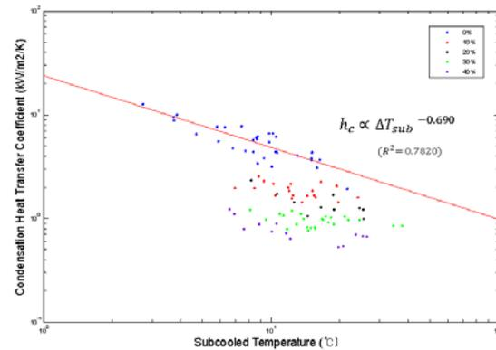
Fig. 5. Condensation heat transfer coefficient of FWC
