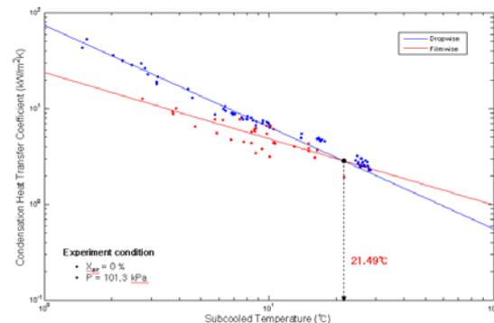
Fig. 6. Comparison of Condensation heat transfer coefficient between DWC and FWC at pure steam condition
