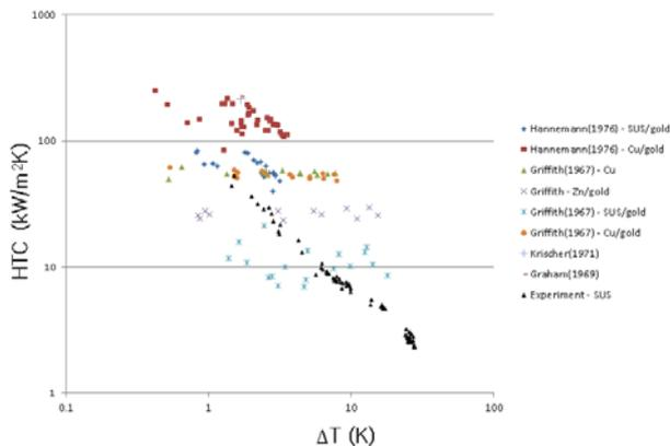
Fig. 3. Subcooled temperature versus HTC of DWC on various cooling surfaces
