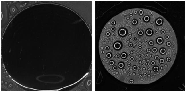
Fig. 2. Condensation surface of filmwise and dropwise condensation
