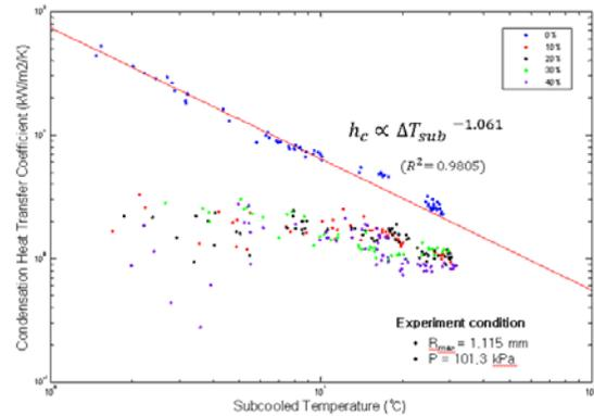
Fig. 4. Condensation heat transfer coefficient of DWC
