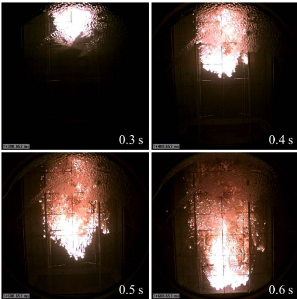
Fig. 2 High-speed camera image of a corium melt jet [2].
