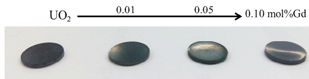
Fig. 1 Photograph of Gd doped UO 2 pellets contain 0, 0.01, 0.05 and 0.10 mol% of Gd, respectively.
