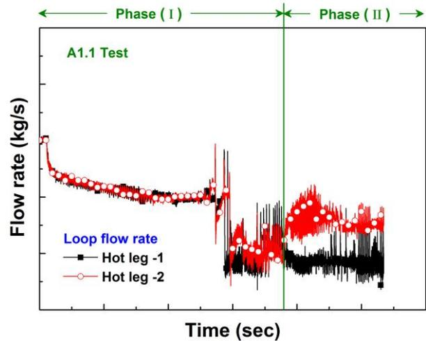
Fig. 2. Flow rates in the hot legs
