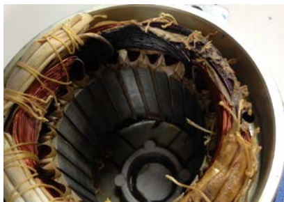
Fig. 13 Windings of a motor after burnout
