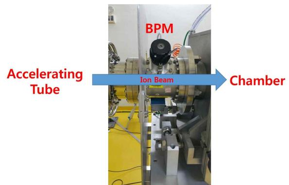
Fig. 1. Installed BPM at the end of the accelerating tube. Ion beam move to right direction.
