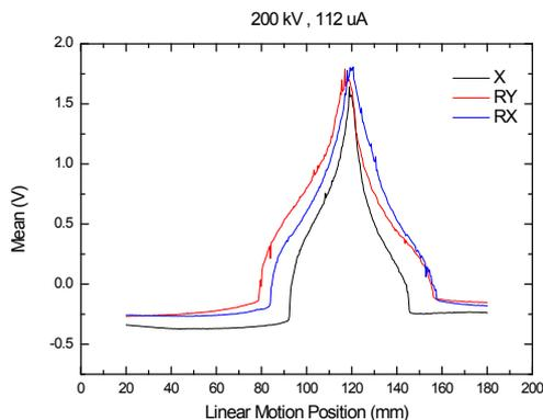
Fig. 4. Beam profile measurement by using wire scanner.
