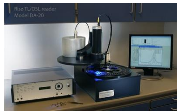
Fig. 1 An automated TL/OSL measurement system having reference irradiator (Risoe Model DA-20)
