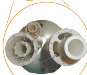
Thermopiles with inconel block removed, as viewed from the top
