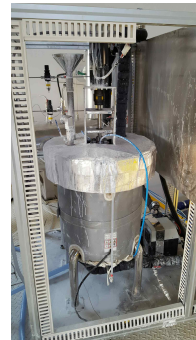
Fig. 4. Aerosol generation and feeding system installed at aerosol scrubbing test loop.
