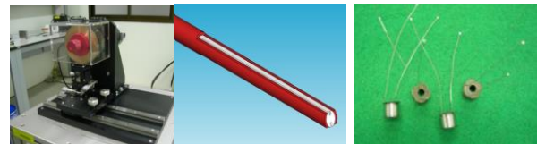
Fig. 4. MI Cable Stripping (Left) and Winded Coils on Bobbin (Right)
