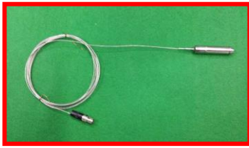
Fig. 5. Final Fabricated LVDT that MI Cable is connected to Miniature Connector.
