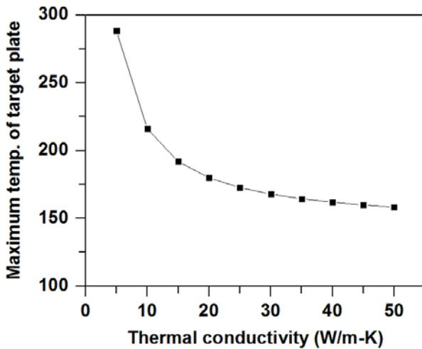
Fig. 3. Maximum temperature of target plate depending on thermal conductivity of  $UAl_x-Al$  target meat.
