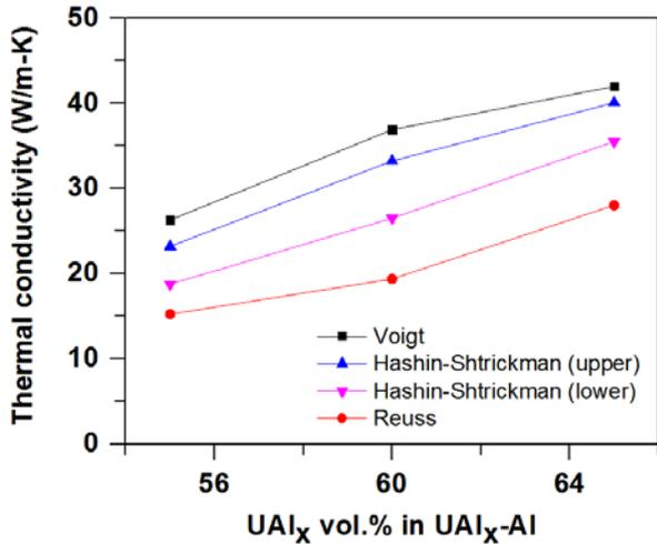
Fig. 2. Effective thermal conductivity of  $UAl_x-Al$  target meat, which estimated using Voigt-Reuss and Hashin-Shtrickman models.
