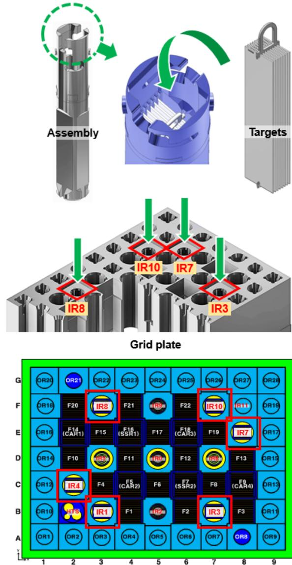
Fig. 4. Schematic diagram of dispersion target assembly loaded in irradiation holes of KJRR
