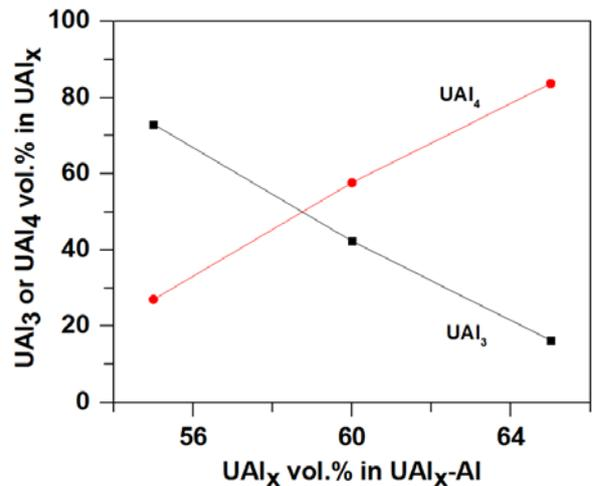
Fig. 1. Volume fraction of UAl<sub>3</sub> or UAl<sub>4</sub> in UAl<sub>x</sub> phase, which result in volume fraction of UAl<sub>x</sub> in UAl<sub>x</sub>-Al target meat.
