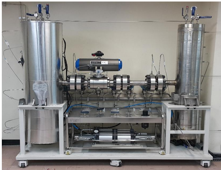
Fig. Experimental Facility for CO 2 leak simulation
