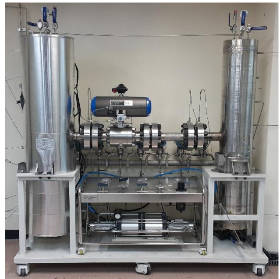
Fig. 4. Designed experimental facility for the CO 2 leak test
