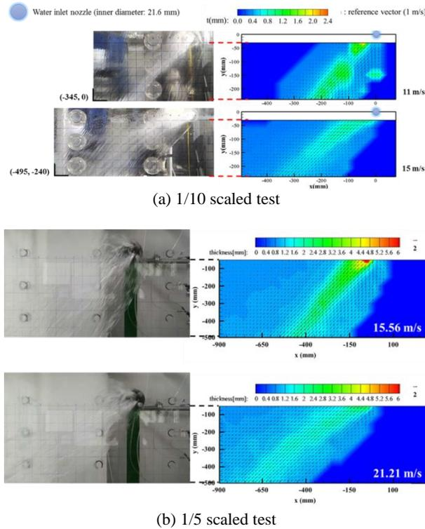
Fig. 2. Local liquid film velocity and thickness
