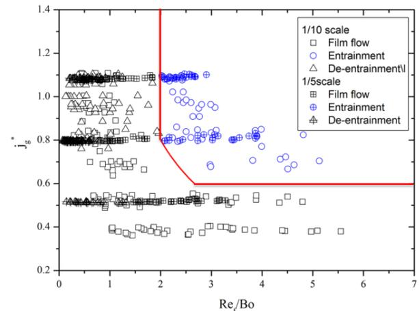
Fig. 3. Onset of entrainment with  $j_g^*$ ,  $Bo$  and  $Re_f$
