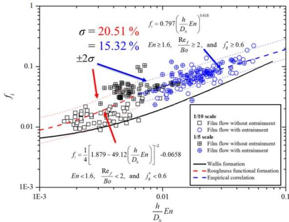
Fig. 5. New interfacial friction model with  $En$
