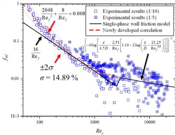
Fig. 4. Wall friction factors and new wall friction model
