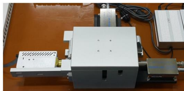
Fig. 2 The prototype of hybrid L-edge/XRF (HLED) system.
