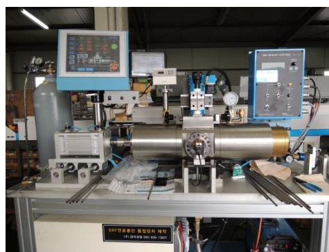
Fig. 2. Photograph of the GTAW system for end plug welding.
