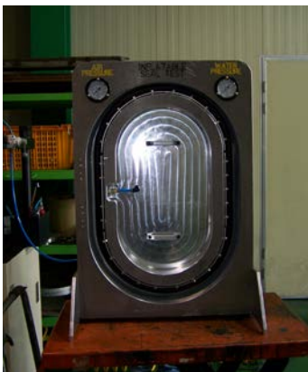
Fig. 4. Test of inflatable gasket
