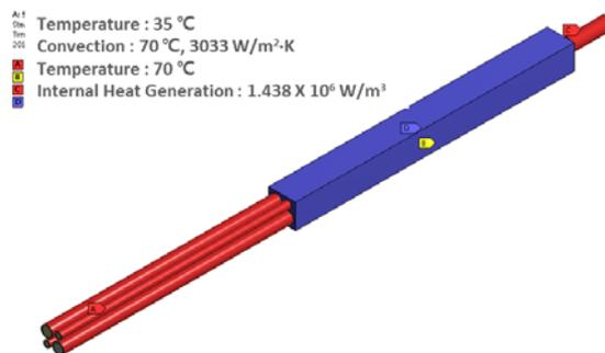
Fig. 2. Boundary Conditions on the FE Model
