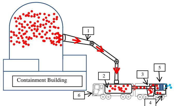
Figure 1. The Configuration of the Integrated Portable Suction-Centrifugal Filtration System
