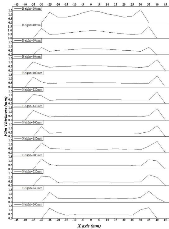
Fig. 1. DVI Liquid Film Flow with No Air(water:0.45m/s)
