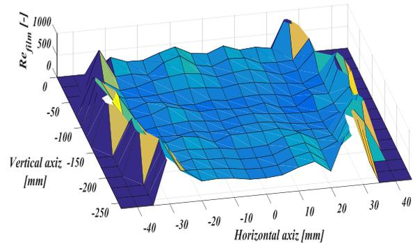
Fig. 7. 2-D film Reynolds number at the water velocity 0.45m/s and the air velocity 0 m/s
