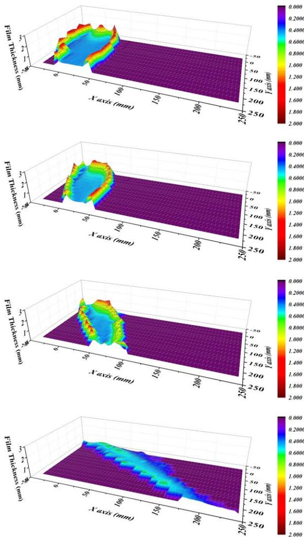
Fig.2-6. Average Liquid Film Thickness obtained by measuring the liquid film flow generated at the water flow rate of 0.45 m/s and the air flow rate of 0, 3, 5, 7, and 9 m/s, respectively.
