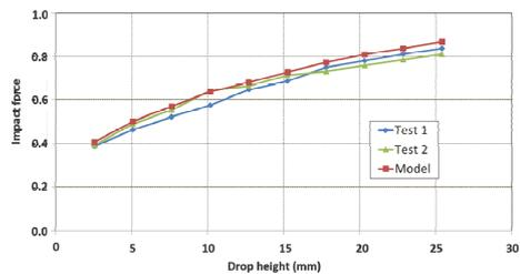
Fig. 7 Axial impact on bottom nozzle
