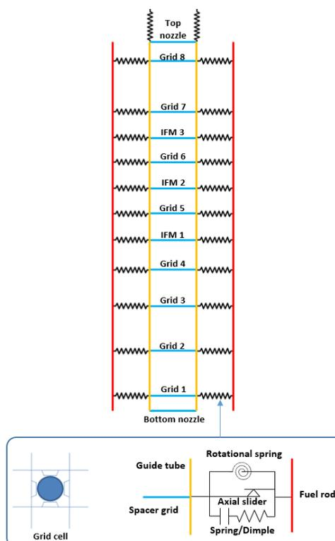
Fig. 1 Fuel assembly finite element model
