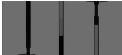
Fig. 2. X-ray radiography image for sodium defect inspection (fuel slug position, sodium level, and top-end plug check; from left to right).
