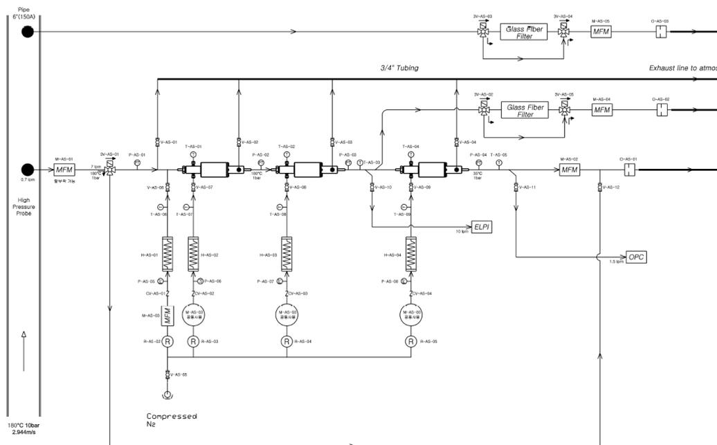
Fig. 3. Aerosol measurement system (inlet)
