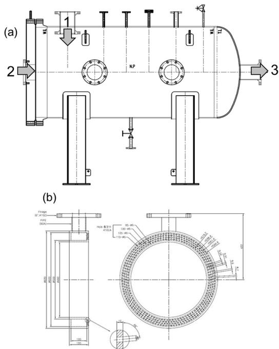
Fig. 2. Mixing chamber structure and distributor. (a) mixing chamber (b) distributor
