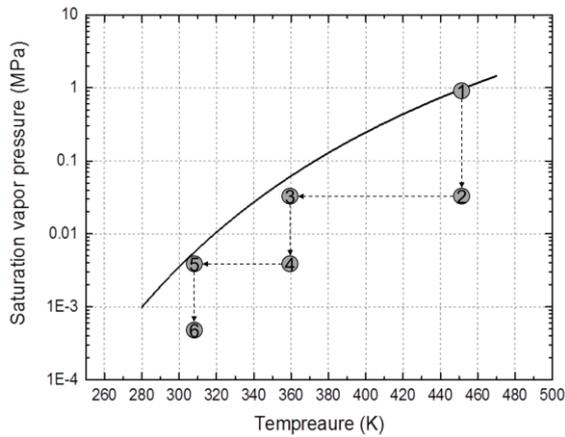
Fig. 4. Temperature and concentration variation of sample gas through diluters
