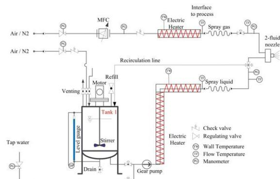
Fig. 1. Aerosol generation system
