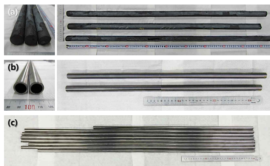
Fig. 3 Outward appearances of (a) hot extruded rods, (b) mother tubes, and (c) thin-walled tubes of ARROS.
