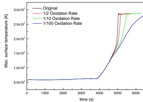
Fig. 1. Maximum cladding temperature according to the reduced oxidation rate for the SBO scenario of PWR.
