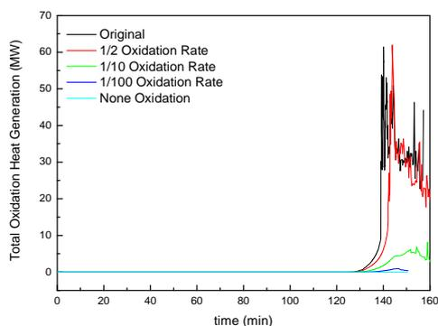
Fig. 2. Total oxidation heat generation according to the reduced oxidation rate for the TMI-2 accident scenario.
