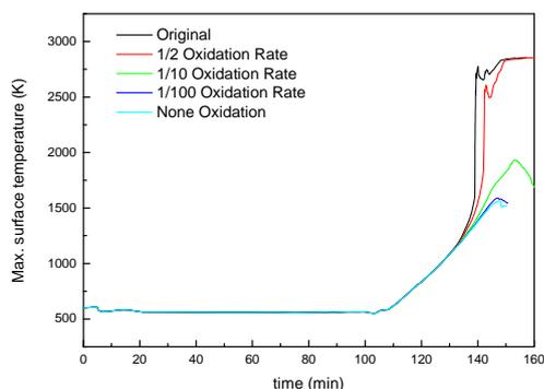
Fig. 3. Maximum cladding temperature according to the reduced oxidation rate for the TMI-2 accident scenario.
